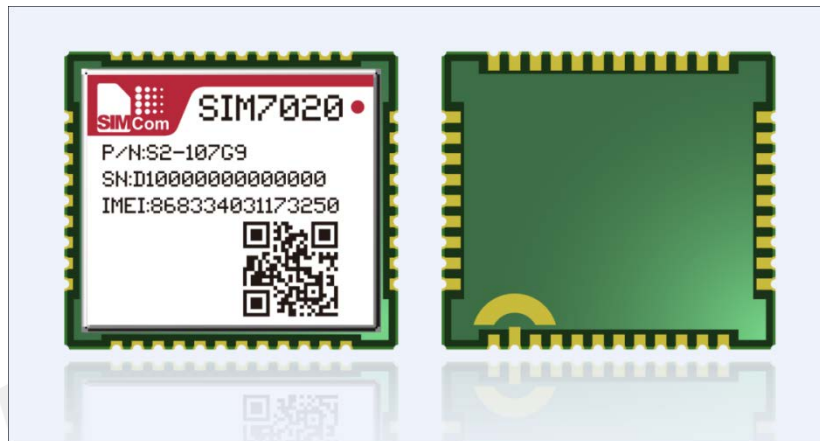
Figure 28: Top and bottom view of SIM7020
