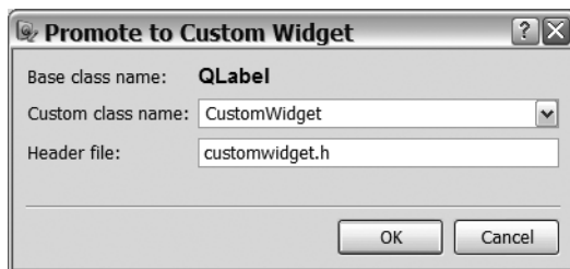
Figure 6-7. Promoting a QLabel to a ClockWidget
