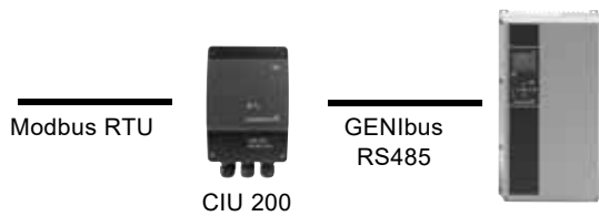
Fig. 2 Principle sketch of CIU 200 Modbus RTU solution. The figure shows a CUE-drive for pumps
