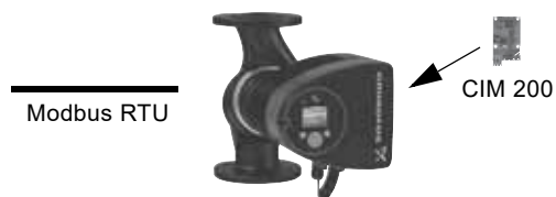
Fig. 1 Principle sketch of CIM 200 Modbus RTU solution with add-on CIM module installed inside the pump. The figure shows a MAGNA3 pump
