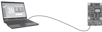
Fig. 20 CIM 500 connected to a PC via ethernet cable
